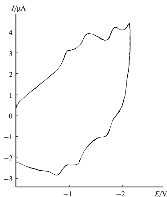
Fig. 3. Cyclic voltammograms of the reduction of diastereomer 1 ( c = 5 \cdot 10^{-4} \text{ mol L}^{-1} ), carbon glassy electrode, o -C 6 H 4 Cl 2 , 0.1 M Bu 4 NPF 6 , potential sweep rate 200 mV s -1 .
